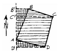
Thus, to obtain the area of the traverse, divide the sum of the double areas by two. For the side AB, the latitude AB' is a + latitude and (B'B+C'C)xAB' is twice the area of the triangle AB'B.
